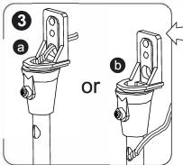
FOR LOUDSPEAKERS WITH KEYHOLE TYPE FIXING Secure universal bracket(h)to upright pole using screw(i). The speaker cable should be threaded through pole and bracket as shown in fig 3a. Or 3b. Assemble thumbnut(t)washers(s)and M4
