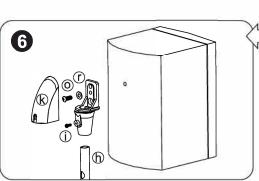
BOSE ACOUSTIMASS LOUDS PEAKERS Attach universal bracket(h) to pole using screw (i) Feed cable down pole as shown in fig 3a or 3b. Attach loudspeaker to bracKet using screw (o) and washers (r).
