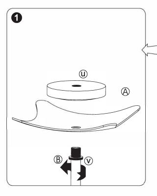
Insert assembled tube (B) into base (A) and screw
